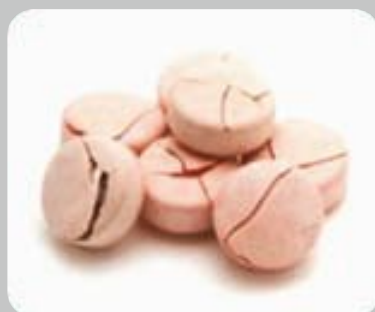
Example of Bad Tablet Coating
